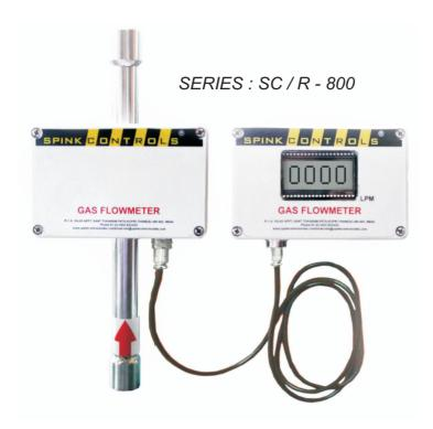
Spink Controls Gas Flowmeter specifically designed to measure the flow of clean gases non-corrosive to silicon. The physical pressure is measured to piezoresistive pressure sensing element where the pressure is converted into a differential voltage signal which is almost proportional to the pressure. This differential voltage is corrected and conditioned in multiple steps, and derive the flow of the gas.
