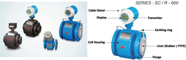
Spink Electromagnetic Flowmeter-Instrument designed for measuring and indicating flow and total volume of conductive liquids. As there are no moving parts in the flow profile the device can be used to measure extremely dirty liquids containing solids. The flowmeter is for use with conductive liquids only. Range of applications. The flowmete has been designed for use in all process industries including chemical, water and wastewater.
