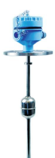
Float Level Transmitters are ideal for continuous Level monitoring in Water, Diesel, Chemical and Oils for accurate level Measurement. The Output is not affected by liquid type, temperature, Pressure and other physical parameters. The Transmitter is factory calibrated and is ready to use.
